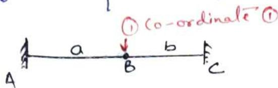
$K_{11}$  = force at ① to produce unit displacement at ①
