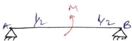
$$\theta_A = \theta_B = \frac{Ml}{24EI} \quad \left| \begin{array}{l} M_{fab} = M_{Fba} = \frac{Ml}{4} \end{array} \right.$$
