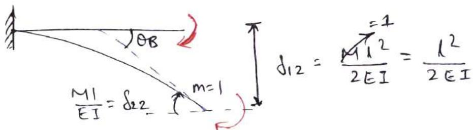
$\delta_{22}$  = Displacement at ② due to unit force at ②
