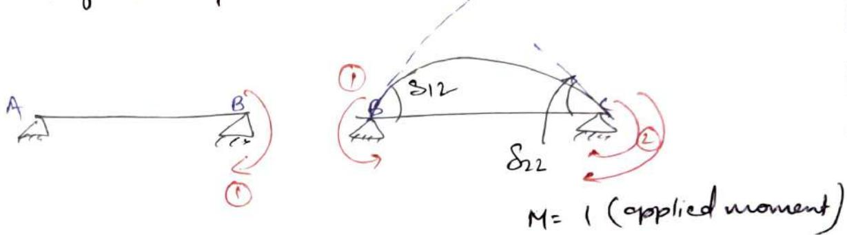
$\delta_{12}$  = Displacement at ② due to unit force at ①
