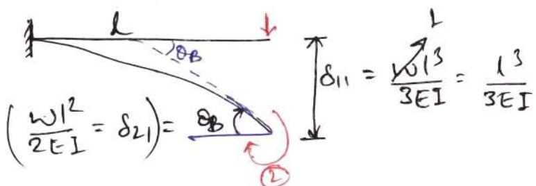
$$\delta_{11} = \text{Displacement at ① due to unit force at ①} = \frac{wI^3}{3EI} = \frac{l^3}{3EI}$$
